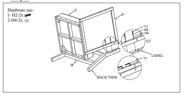
Position Backrest (D) onto the Right Leg Frame (B) ensuring all labels match (E with E) as illustrated. Align holes in Backrest (D) with holes in Right Leg Frame (B). Secure connections with Allen Bolts (H-2) with provided Allen Key (T-1). Do not fully tighten until all hardware has been engaged.
