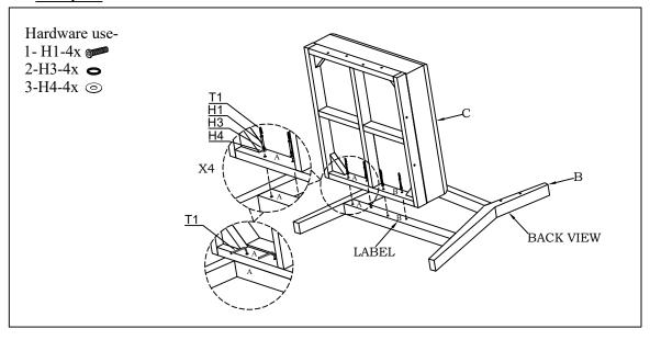
Place Right Leg Frame (B) down onto a padded, non-marring surface. Position Seat (C) onto Right Leg Frame (B) ensuring all labels match (A with A, B with B). Align holes in Seat (C) with holes in Right Leg Frame (B). Secure connections with Allen Bolts (H-1), Lock Washers (H-3) and Flat Washers (H-4) using provided Allen Key (T-1), stacking the hardware in the order as shown. Do not fully tighten until all hardware has been engaged.
