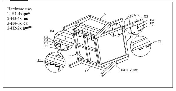
Position Left Leg Frame (A) and repeat steps 1 and 2. Do not fully tighten until all hardware has been engaged.
